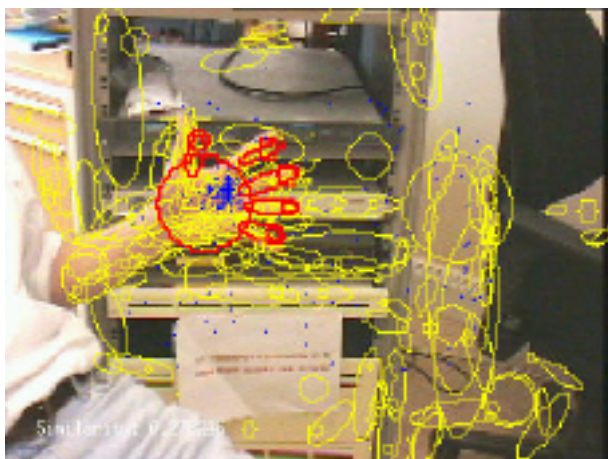
Fig. 1 Detection of multi-scale features in a video stream of a complex scene.
